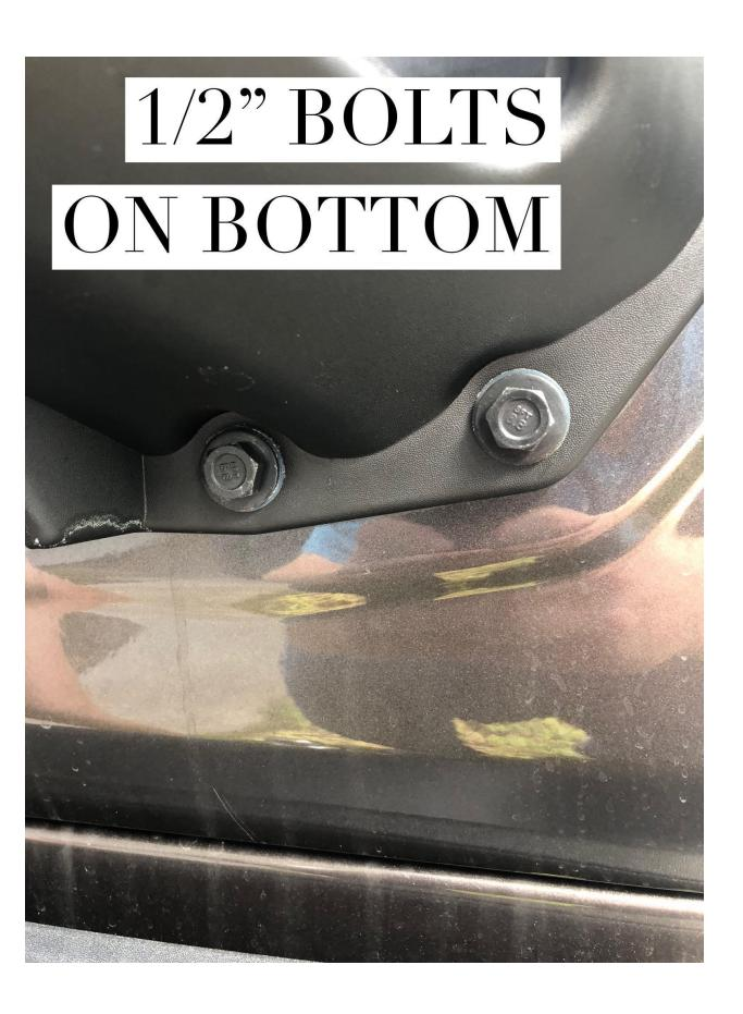
**STEP 5:** Hold up Rough Country bracket and line up the 8 factory holes to the 8 holes on the NEW bracket. Using factory hardware, re-install 8 bolts with deep socket into the new bracket to hold it on. 4 on the top and 4 on the bottom.
