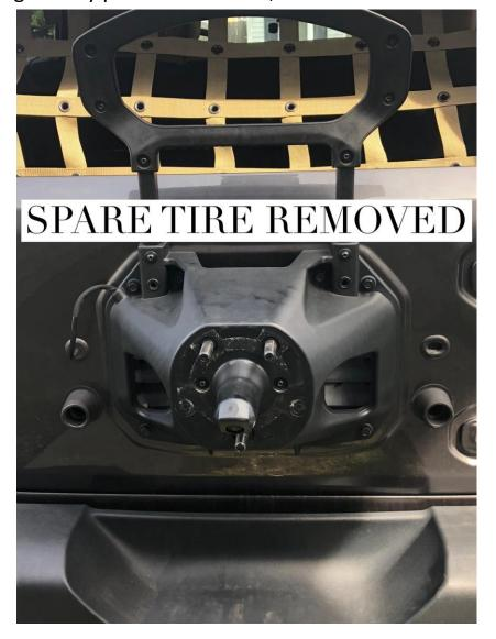
**STEP 2:** Remove the 7 brake light bracket screw and pull apart to separate bracket. Re-route wire inside to provide more length. After moving wire re-install the 7 screws
