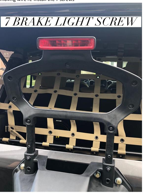
**STEP 3:** Remove the 4 screws that holt the brake light bracket to the spare tire bracket. Move the bracket up by aligning the bottom hole on the brake light bracket to the top hole on the spare tire bracket. Reinstall 1 screw on each side to keep bracket up, leaving top hole on brake light bracket empty. Save other 2 screws as spare parts.
